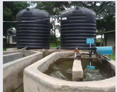
Figure 2: A Pilot-scale HRAP system with and without a paddle wheel at FNRES, Namasagali Campus
