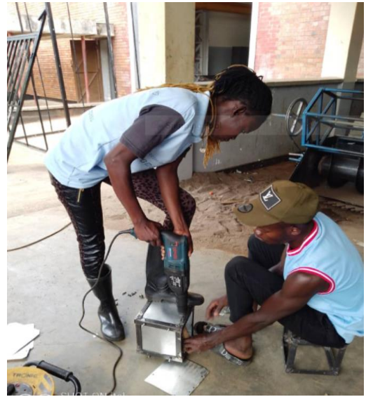
Students fabricating a hopper for the silo
